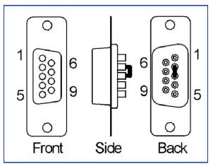
Make a serial loopback connector by soldering pins 2 and 3 together, as shown.
