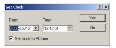
Use a delayed start-up either to make sure the Aquadopp Profiler starts data collection on the hour or to conserve batteries for a deployment that starts some time in the future. You can start an Aquadopp Profiler deployment well in advance of when you plan to install it on site, and use a delayed start-up to conserve the Aquadopp Profiler's battery and recording resources for the actual deployment.
