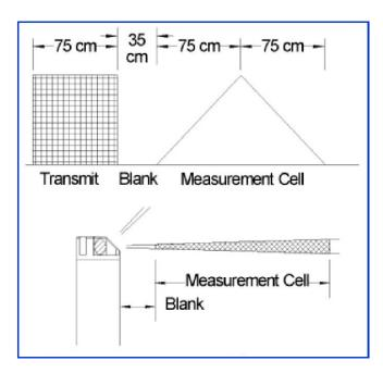
*Measurement cell location.* The 75 cm dimension that applies to the transmit pulse and measurement cell is fixed by the Aquadopp software, but you can adjust the blank. Given the default 35 cm blank, the center of the measurement cell is located at 110 cm (=35+75) from the sensor head.
