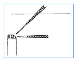
When the Aquadopp Profiler is near a boundary, avoid letting the measurement cell touch the boundary.
